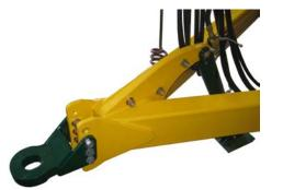
When hitching cultivator to tractor drawbar use the largest pin possible.
