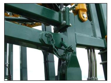
Pin Locked in Transport Position
